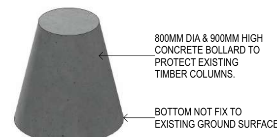
CONCRETE BOLLARD FOR COLUMNS 3D
