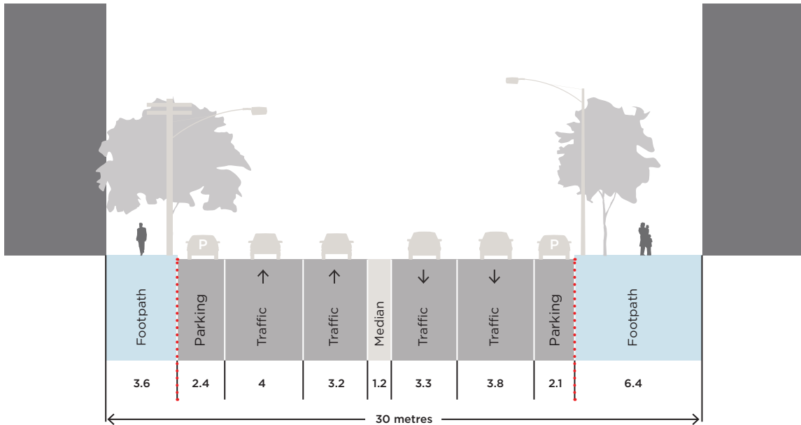
Figure 3.18: Existing conditions of City Road between Queens Bridge Street and Balston Street, looking east towards Power Street (Section B)
