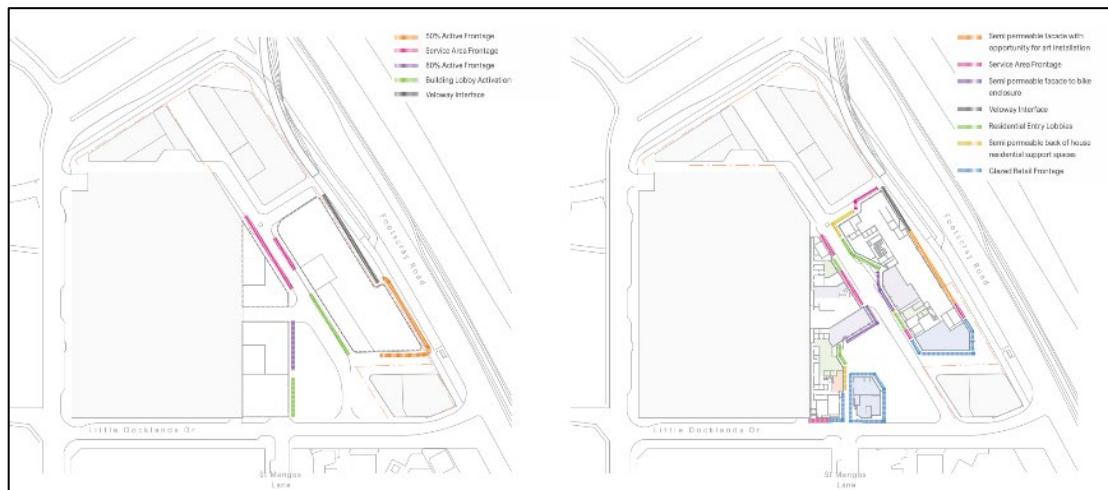
Figure 19 - Activation requirements of the development plan (left image) compared to proposed levels of activation (right image) (source: Urban Context Report)
