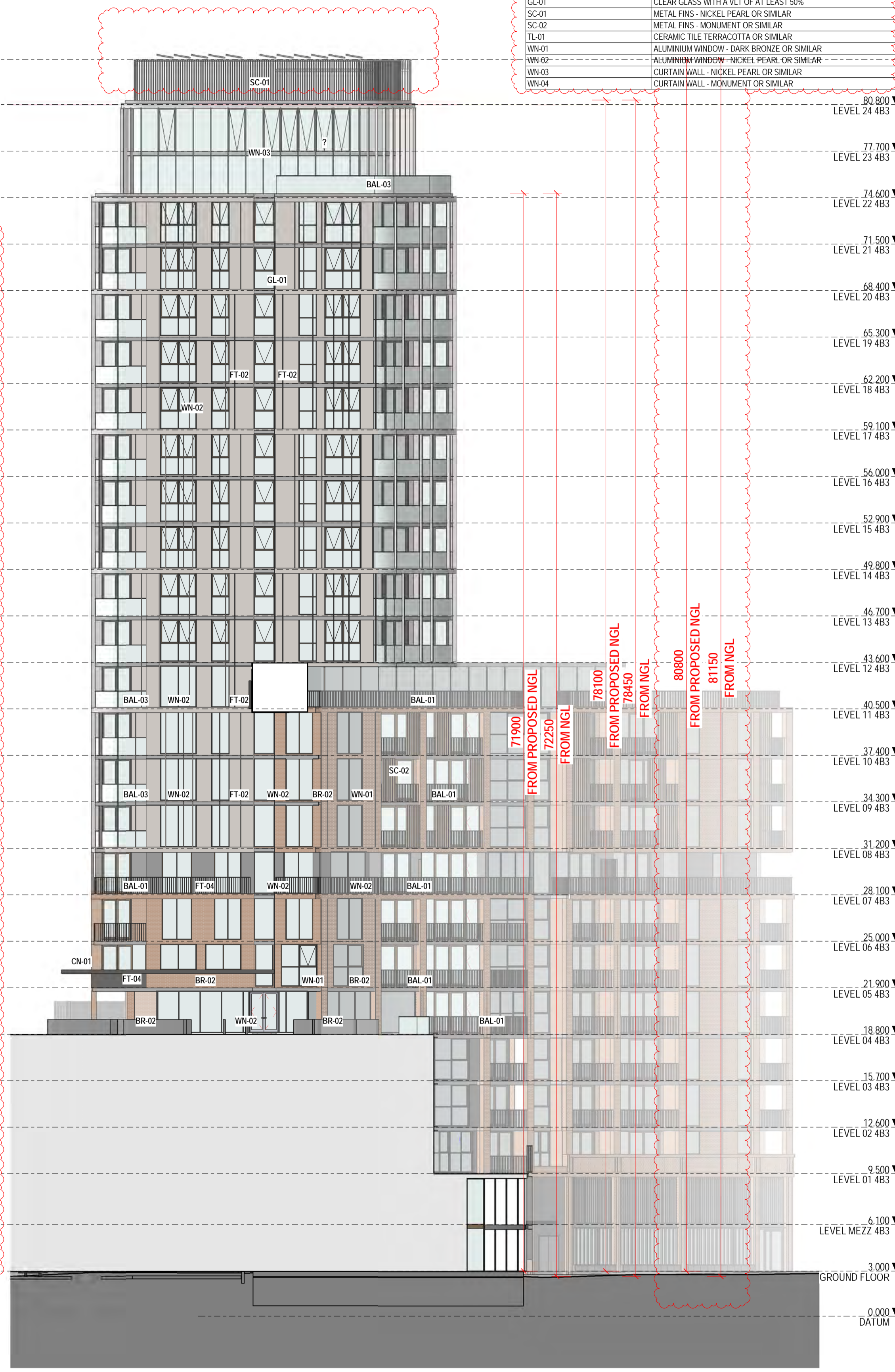
4B3 - SOUTH EAST ELEVATION - NORTH TOWER 1 : 200
