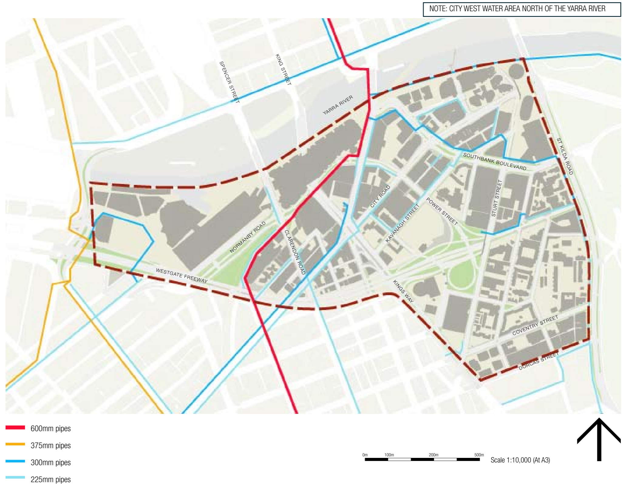
Fig 4.4.1 Water Supply Locations
