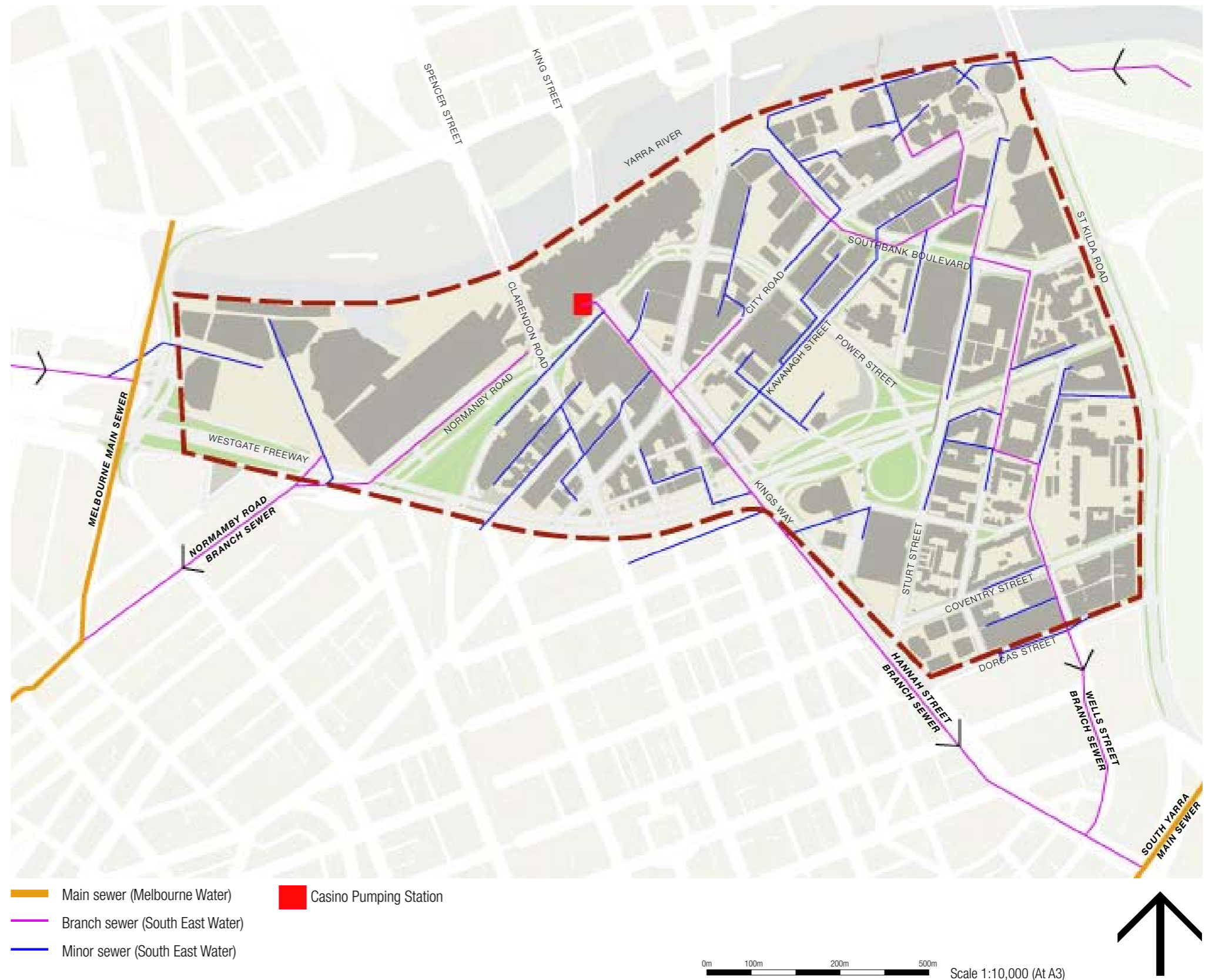
Fig 4.5.1 Sewer Pipe Locations
