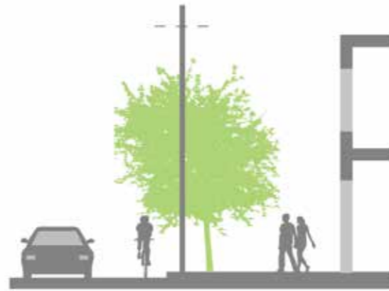
Small tree under powerlines
