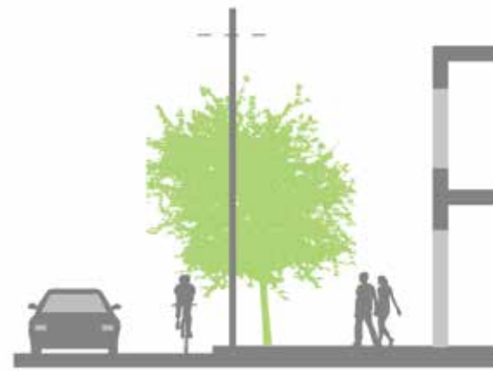
Small tree under powerlines
