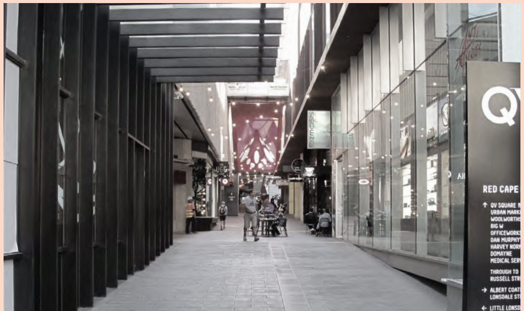
Figure 49 Canopies that cover the majority of a laneway reduce the sense of openness and publicness, while obscuring any visual connection to upper levels.
