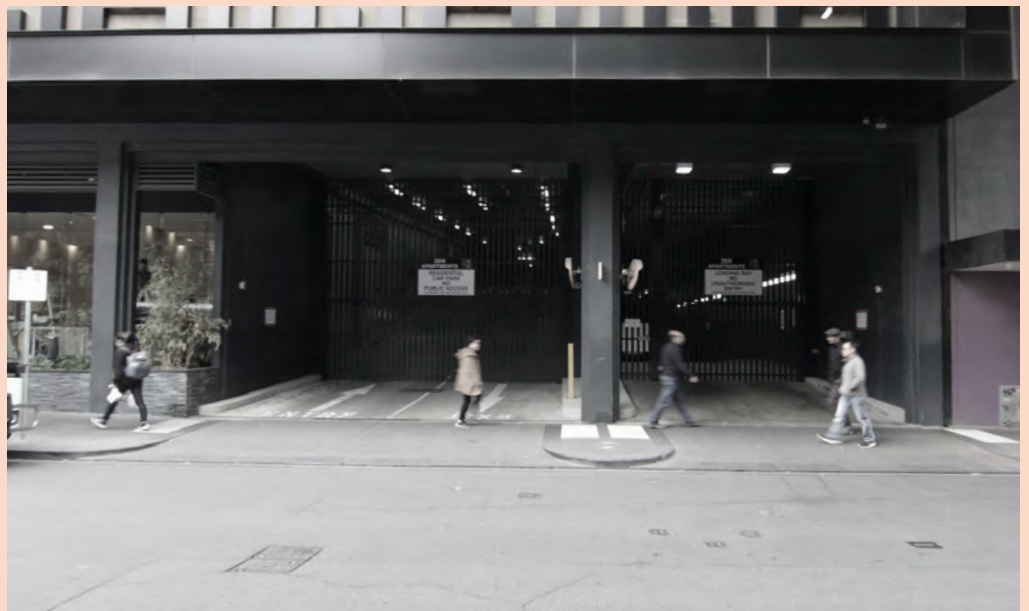
Figure 38 A deep setback to the carpark access door results in an undesirable space which feels unsafe at night and impacts the continuity of the pedestrian realm.
