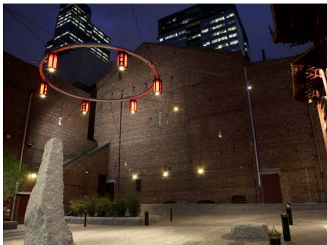
Image 18. Cohen Place, in Chinatown. Even in an area with decorative lighting, most light is directed to the pavement and facade lighting is carefully directed to avoid spill. Full details can be found in Appendix 3 - Photo References.
