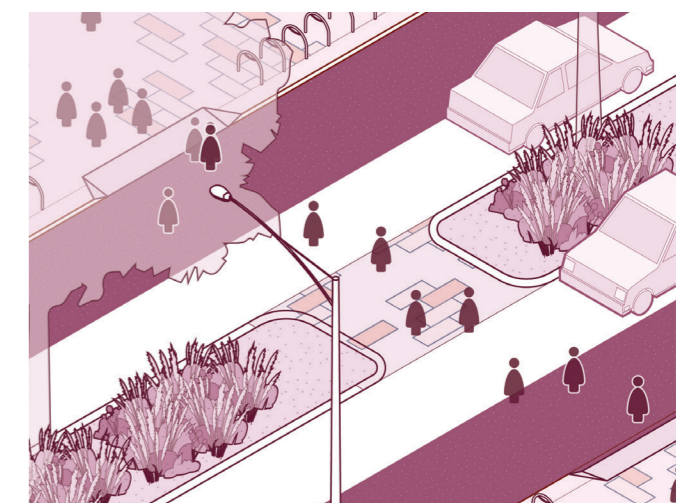
Figure 34: Mid-block crossing points
