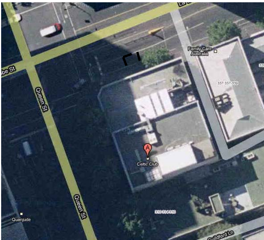
Figure 3 Aerial view of building, showing added service platforms over the light court (Google Maps)
