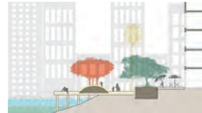
Planting on structure: trees growing on mound to achieve required soil volume for tree planting
