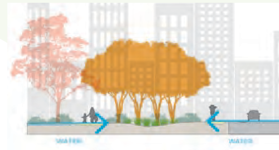
Water infiltration, permeable paving and structural soil or cells provide opportunities to grow larger, healthier trees in paved areas.
