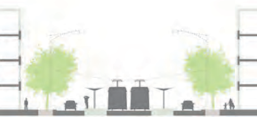
Tram infrastructure prevents median tree planting, and overhead services clearances influence tree placement in footpaths
