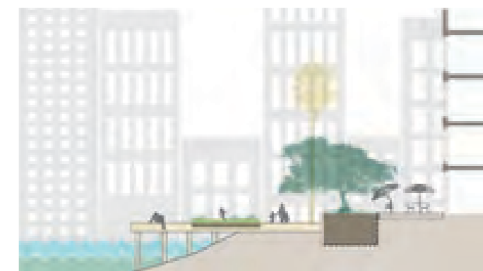
Planting on structure: garden bed with required soil volume for ground cover planting.
