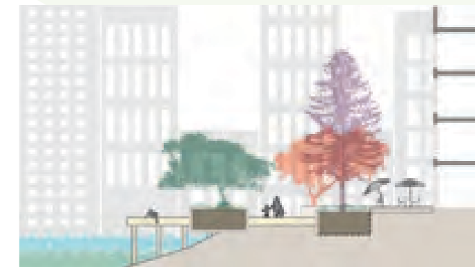
Planting on structure: raised garden bed to achieve required soil volume for tree planting
