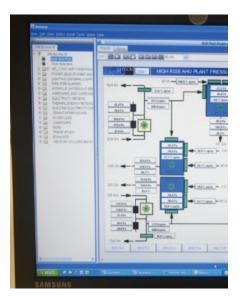
Key sensors to the control systems (supply air temperature and system pressure) were recalibrated and relocated to improve reliability and accuracy.
